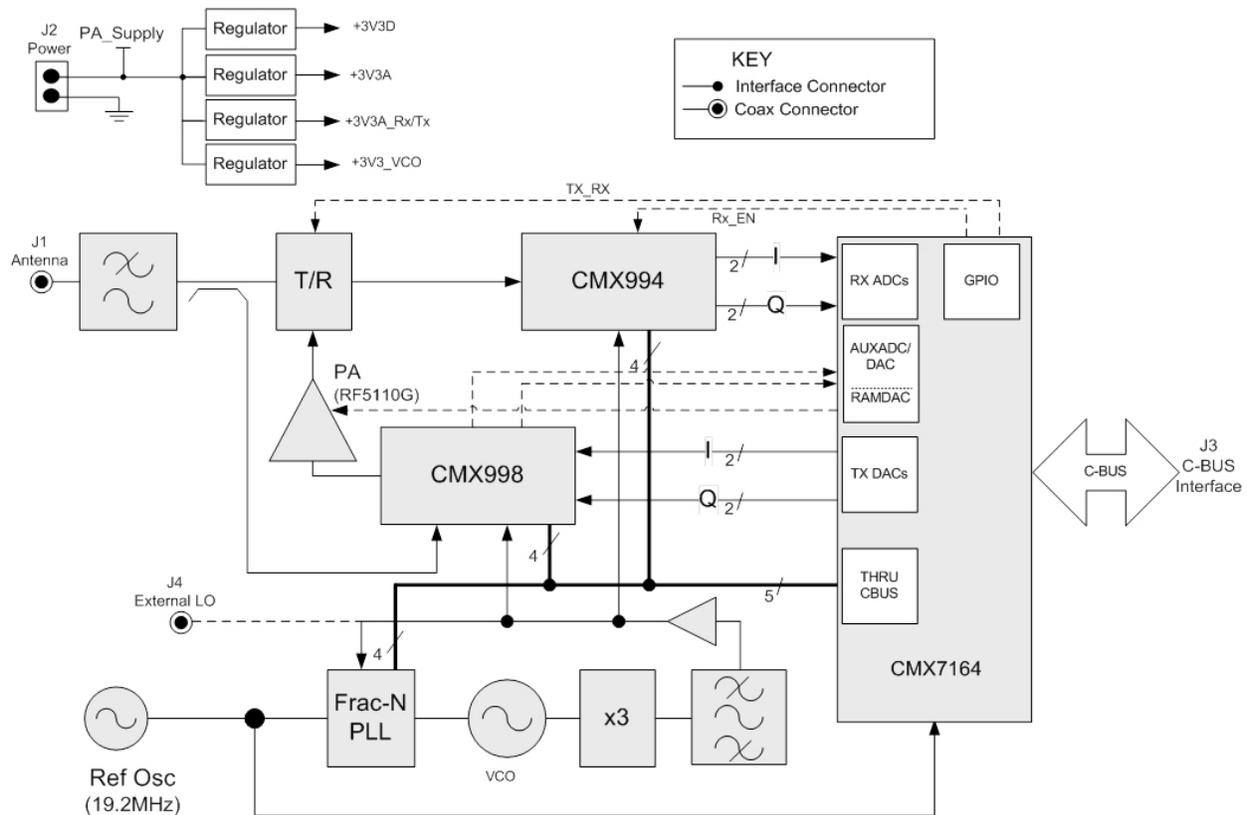
Figure 1. DE9941 Demonstrator Board Block Diagram
